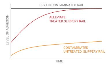
The graphic on the left depicts the very low levels of adhesion typically observed with wet, slippery rail. These low levels of adhesion can result in very poor traction.
