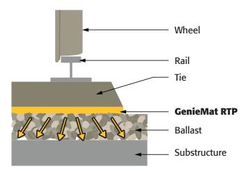
**GenieMat RTP** Railway Tie Pads protect track components by reducing impacts and dispersing load over a greater area of ballast.
